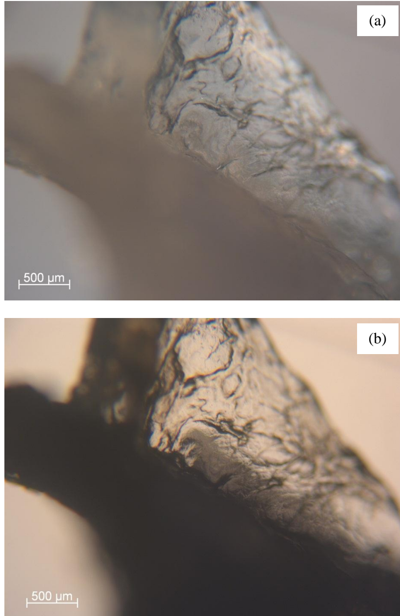
Figure 5.21 Polarized light microscopy of remaining 30ASP10HT after 48 hours of dissolution in pH 7.4 medium (a) 75° position (b) 0° position.
